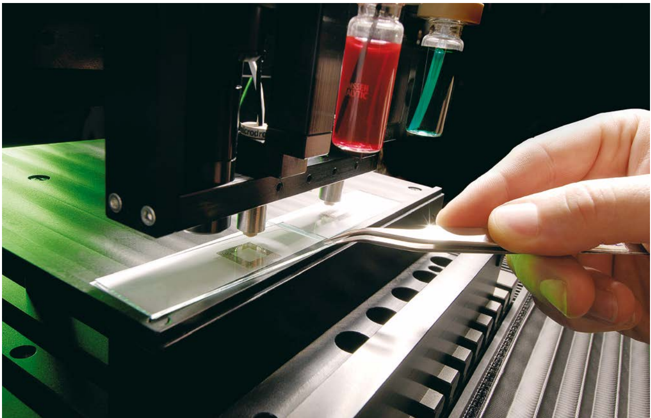
Sample production with Printing System Autodrop Professional AD-P-8000
